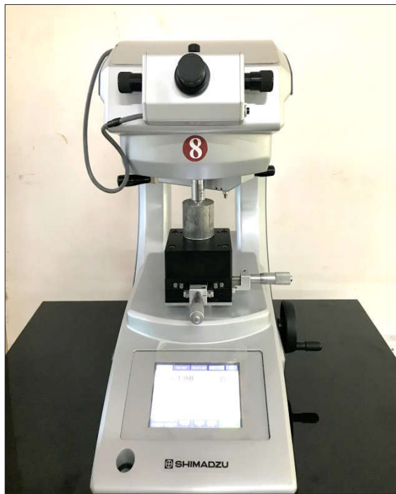
Fig. 2. Specimen loaded on (Shimadzu) hardness tester
