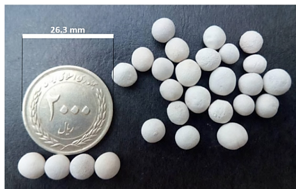
Fig. 1. Calcined granules (70% kaolin, 30% gibbsite).
