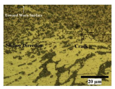
**Fig. 4.** Optical Micrograph of subsurface of worn specimen at 100N showing plastic deformation in the direction of sliding. The arrows indicate the cracks in the subsurface, and the circle suggests Al-Si eutectic led to crack deflection.
