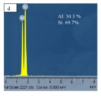
Fig. 3. (a) and (c): SEM secondary electron images of the alloy as-cast and T6 treated; (b) and (d): EDS spectrum of the eutectic compounds of the alloy as-cast and T6 treated
