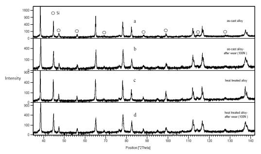
Fig. 1. X-ray diffraction patterns of the alloy: (a) before wear (b) after wear (100N) (c) heat treated alloy (d) heat treated alloy after wear (100N).
