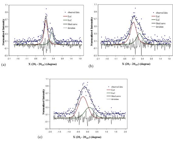
**Fig. 2.** The measured and the fitted curve via Pearson function corresponding to the 400 reflections of Al: (a). before wear (b). 100N (c). 150N, the difference between the measured and the fitted values is also plotted in the lower parts.
