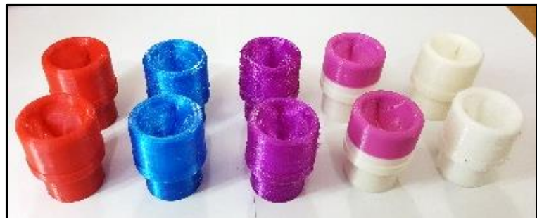
Fig. 10. The 3D printing of artificial tri-leaflet heart aortic valve (TAV) mechanical heart valve
