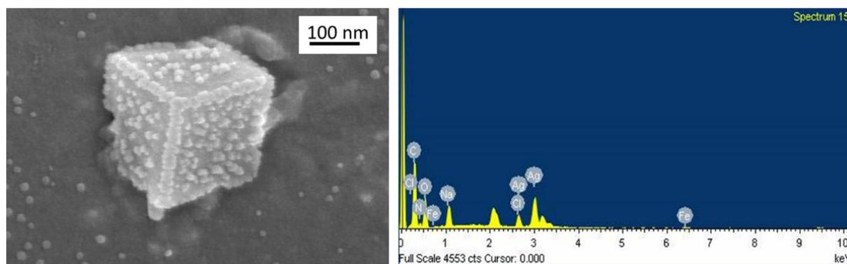
Fig. 5. Elemental analysis of nano-Ag confirmed by EDX.
