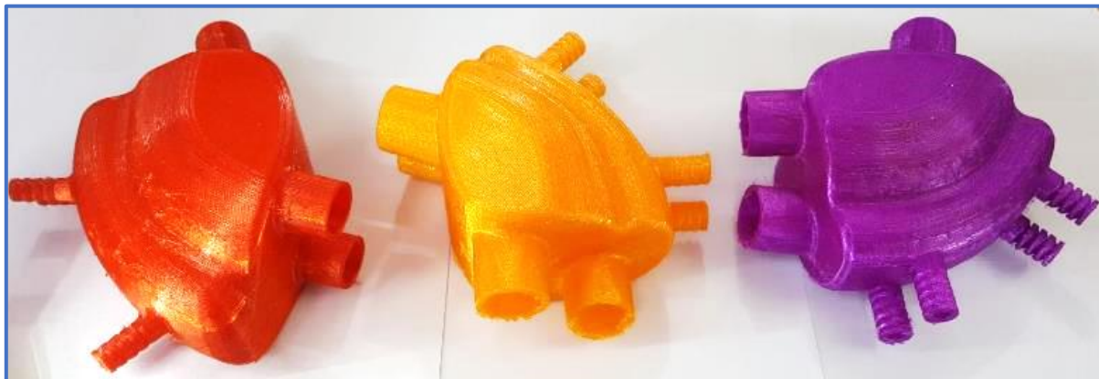
Fig. 11. The final 3D print of the designed total soft artificial hearts from a red TPE, and the transparent orange and purple TPU filaments materials, respectively.
