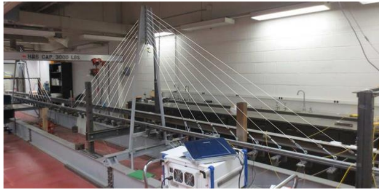
Figure 13: Laboratory Cable-Stayed Bridge [27]
