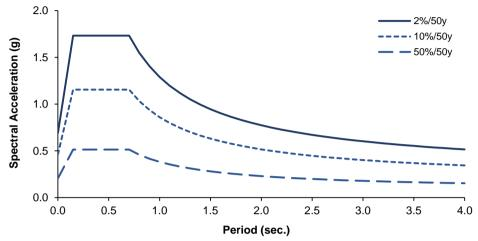
Figure 1. Acceleration response spectra of hazard levels
