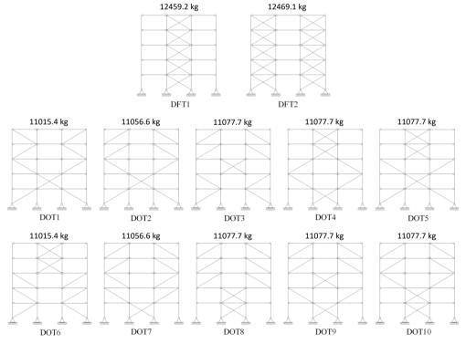
Figure 3. Optimally designed 5-story SCBFs
