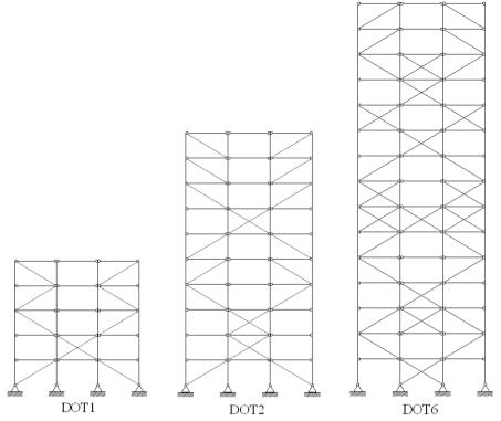
Figure 9. The safest optimally designed 5-, 10- and 15-story SCBFs
