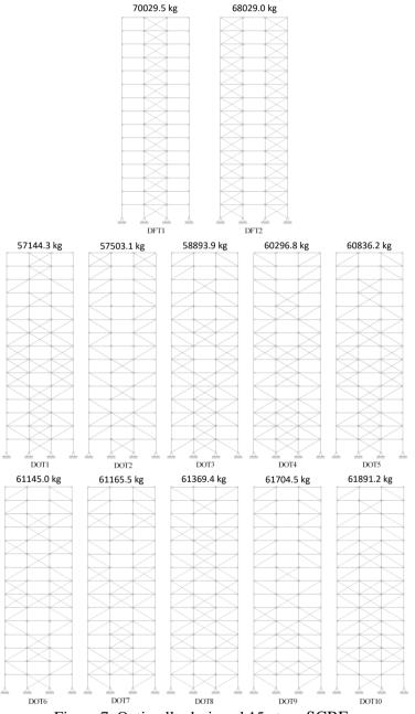
Figure 7. Optimally designed 15-story SCBFs
