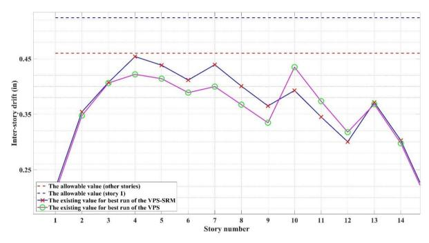
Figure 4. Inter-story drift values calculated at the obtained optimal design by the VPS-SRM and VPS for the 3-bay 15-story frame structure
