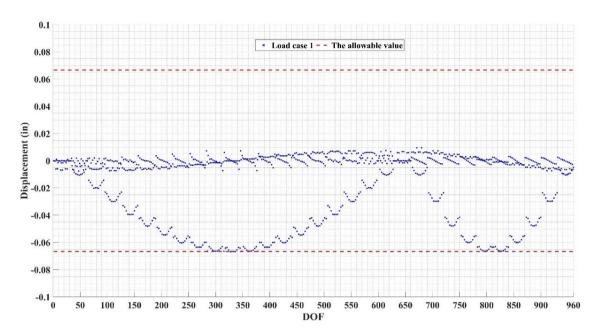
Figure 12. Displacement values found by the VPS-SRM for the 1016-bar double-layer grid.
