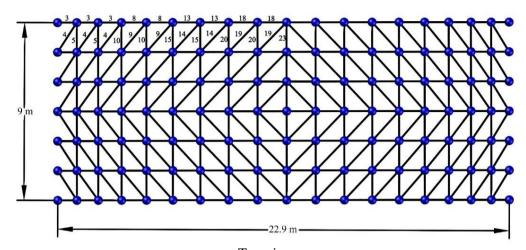
Top view Figure 6. The 693-bar double-layer barrel vault
