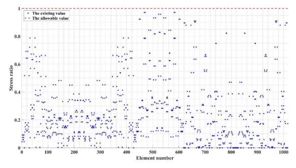
Figure 11. Stress ratios found by the VPS-SRM for the 1016-bar double-layer grid.
