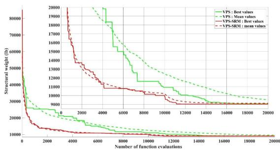
Figure 9. Convergence histories of the best and average of runs for the 693-bar double-layer barrel vault
