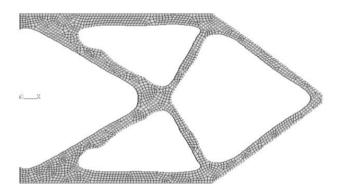
Figure 8. The optimal topology of the cantilever beam [9]
