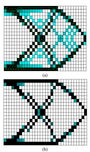
(b) Figure 7. (a) The PGT (shown in green lines) mapped on the density distributed media and discontinuous region (in cyan ink), (b) the model after removing the discontinuous region
