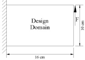
Figure 2. The cantilever beam topology optimization problem under the load (F=500 N) [9].
