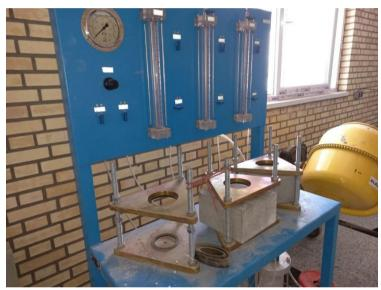
Figure 17 An image of the permeability test apparatus
