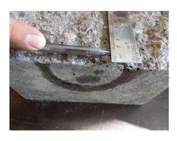
Figure 19 The method of reading the water permeability value after the sample is split
