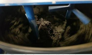
Figure 9. Sample preparation with electric mixer
