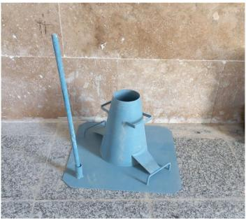
Figure 10. Slump test cone
