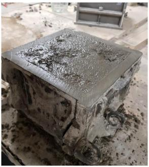
Figure 11. A 150 millimeter mold filled with concrete
