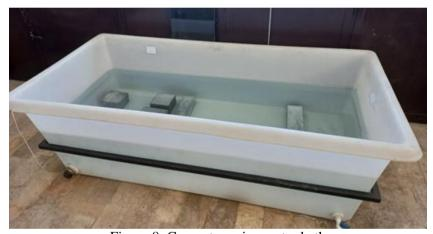
Figure 8. Concrete curing water bath
