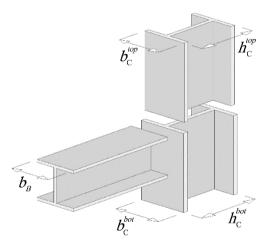
Figure 5. A typical framing joint
