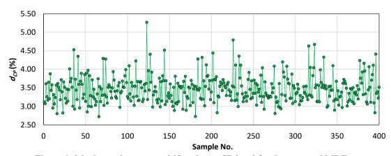
Figure 9. Maximum inter-story drift ratios at CP level for 5-story steel MRF
