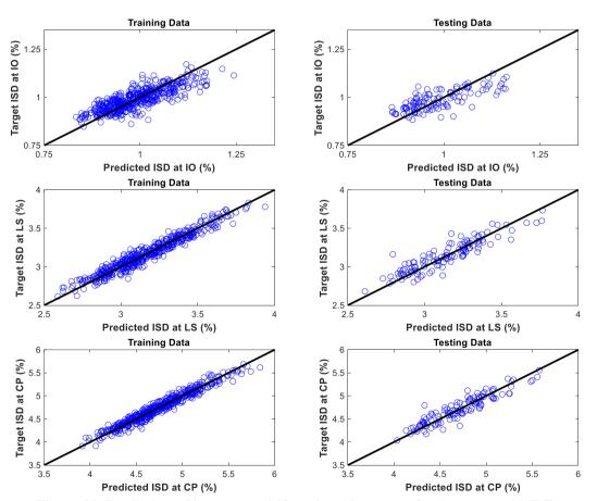
Figure 22. Prediction of inter-story drifts using 10 neurons for 5-story steel MRF
