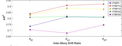
Figure 12. AR<sup>2</sup> of inter-story drift ratios predicted by NN models for 5-story steel SMF
