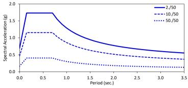
Figure 1. Acceleration response spectra
