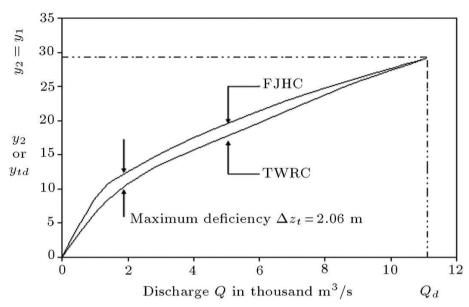
Figure 2. Free Jump Hydraulic Curve and Tail Water Rating Curve for Tehri dam [33]
